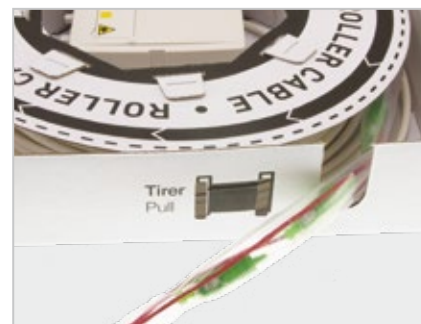
Full connectorized cable pulling
